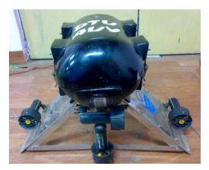
The new mechanical model is designed to be hydro dynamically stable. The vehicle features a seamless, smooth contoured ellipsoidal body. The shape of the vehicle has been decided after calculations, keeping various hydrodynamic parameters in mind to improve the overall
